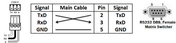
Note: Captive screw connector may also be used as a serial connection.
