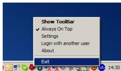
Clicking **Exit** will shut TelRecorder down. No recording is then possible, even when TelRecorder is set to record automatically.
