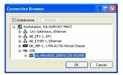
4 A green border around the controller icon indicates that CCW is online with the controller.
