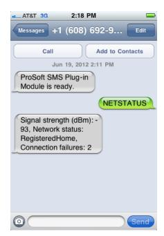
The sample controller program for the ILX800-SMSG plug-in module recognizes the text message commands listed in the following two tables. When the module receives a text message command, it sends a response text message to the originator of the text message command.
