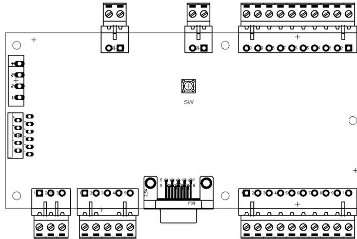
Figure 3.17 Location of the back-up battery power supply switch on the main board.
