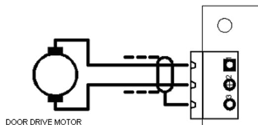
Fig. 6.1 Motor power terminals
