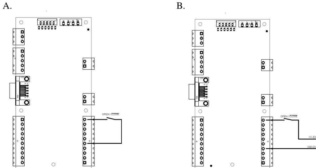
Figure 3.8 Connection of control signals - using OPEN input only
