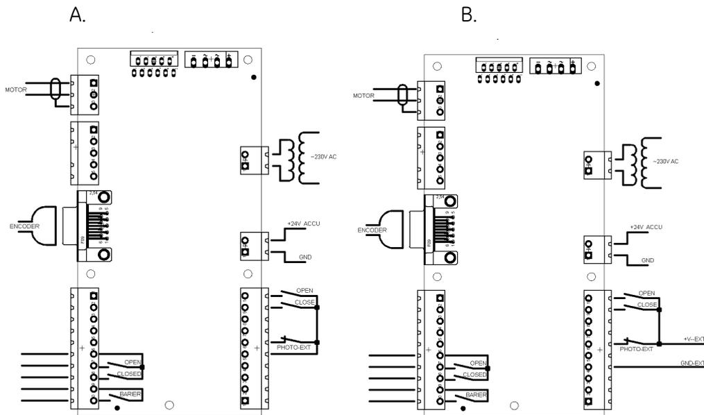
Figure 3.2 Connection options of SDK 250 Controller
