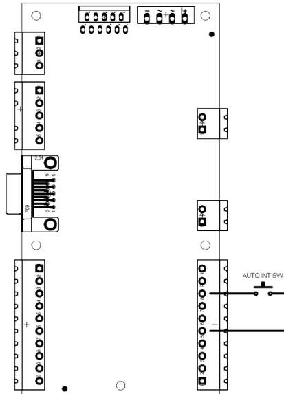
Figure 3.14 Connections of auto initialisation switch to SDK 250 controller.
