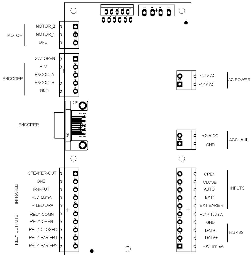
Figure 3.1 External connectors of SDK 250
