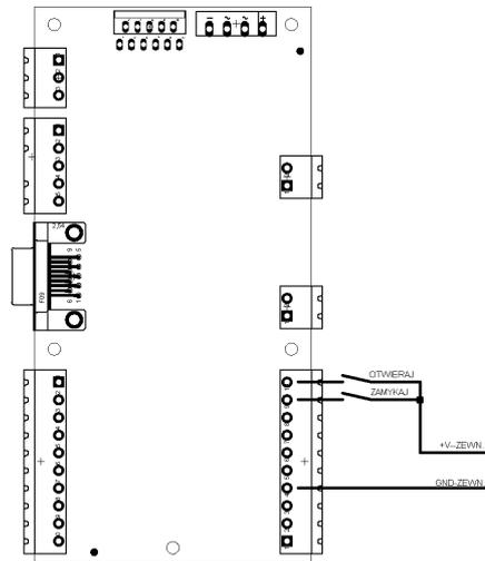
Figure 3.7 Connections of control inputs
