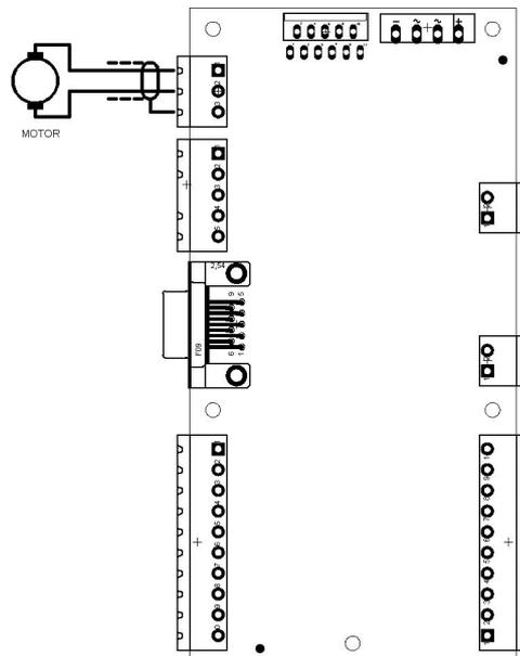
Figure 3.4 Motor connections of the SDK 250
