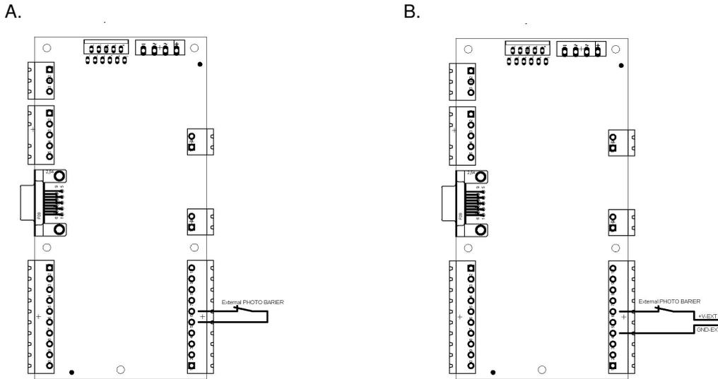
Figure 3.12. Connections of the external optical barrier.
