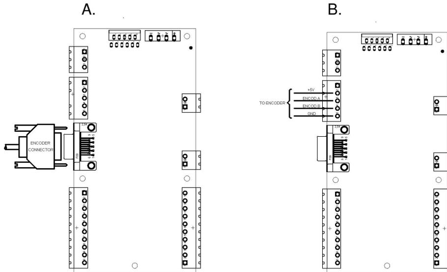
Figure 3.5 Connection of encoder to SDK 250 using DB-9 connector or wire terminals.
