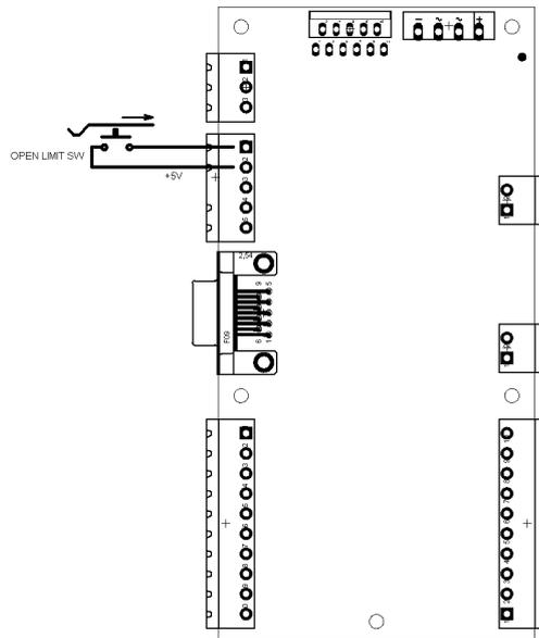
Figure 3.15. Connections of optional terminal position contact – door open.
