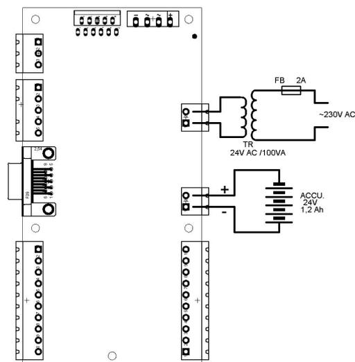
Figure 3.3 Power Supply connections
