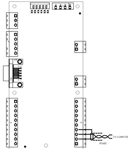
Figure 3.16 Connections of RS 485 communication bus.
