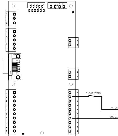
Figure 3.9 Connection of control signals - using CLOSE input only
