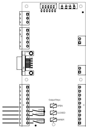
Figure 3.10 Connection of relay outputs of SDK 250 controller.
