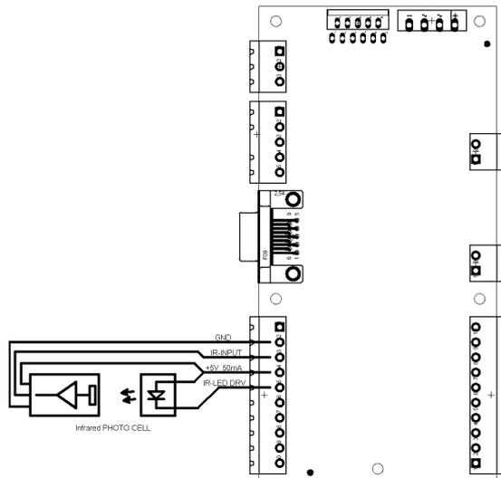
Figure 3.13. Connections of dedicated optical receiver and transmitters to SDK 250 controller.
