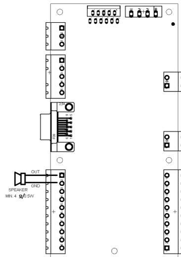
Figure 3.11 Connection of a chime speaker.
