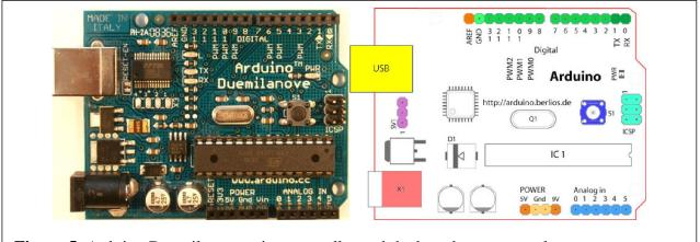
Figure 5. Arduino Duemilanove microcontroller and the board component layout.
