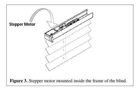
A 5V stepper motor will be used to control the physical movements of the SPSB system. The stepper motor is illustrated in **Figure 4**. Specifications for the stepper motor are described as follow:
