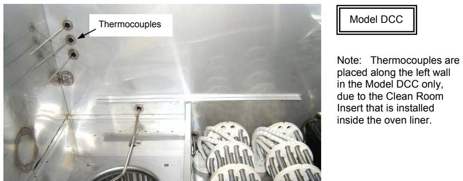
THERMOCOUPLE LOCATION – MODEL DCC
