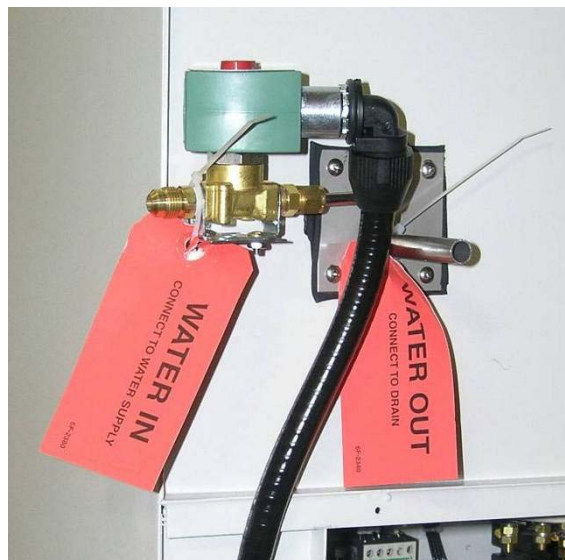
WATER SUPPLY CONNECTIONS
