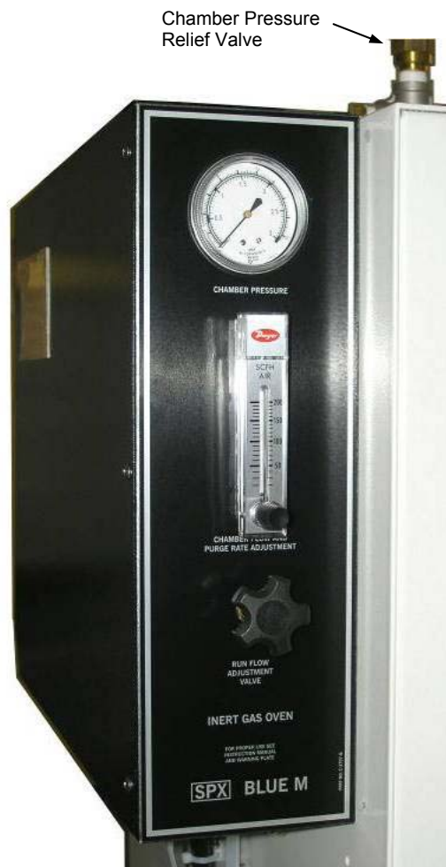
INERT GAS CONTROL SYSTEM
