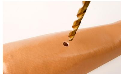
Smooth the edges of the drill hole and insert the threaded charge port. A minimum thread height of 3.2mm above the socket surface is required for full engagement of washers and locking nut.
