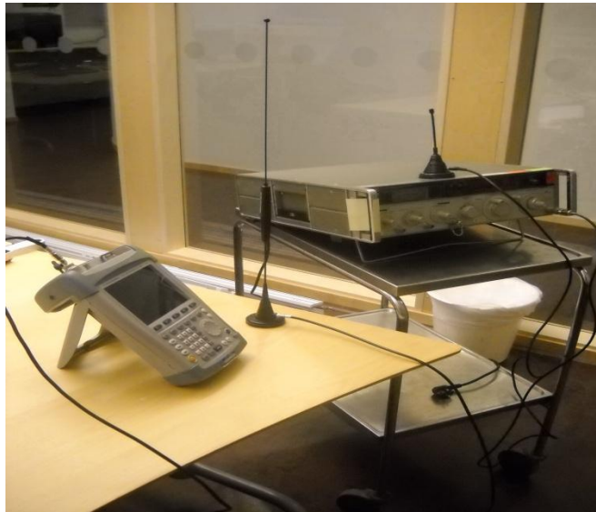
Fig 23: Sample setup for 385MHz measurements
