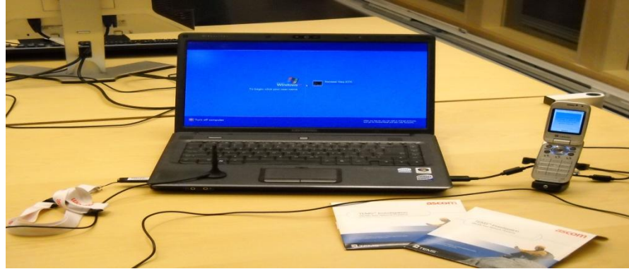
Fig 24: TEMS tool kit interfaced with PC acts as a receiver unit.
