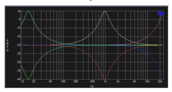
GML8200 band pass section responses, showing full frequency ranges from 15Hz to 26KHz with  $\pm 20dB$  gain ranges.
