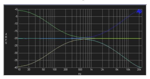
Characteristically gentle GML8200 shelving curves with frequency range to 26 KHz and with full +/- 20 dB boost and cut gain ranges.
