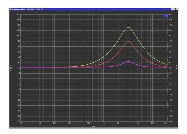
This style has minimal Gain / Q dependency, smaller amounts of boost or cut still have relatively high Q and it is therefore precise and well defined in use.
