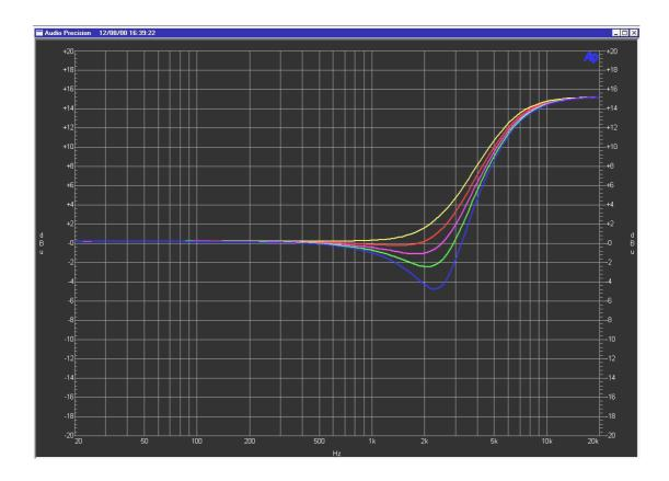
When the HF shelving function is selected, the Q control provides control of the 'overshoot' function.
