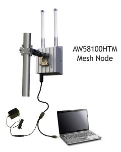
Step 3. The default IP address of the radio is written on its product label. This address is 192.168.88.11 with a subnet mask of 255.0.0.0. You must configure your PC's wired LAN port to the same subnet and an IP address different from that of the radio. With this configuration in place, you should be able to use a web browser on your PC to log in to the radio's interface.
