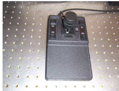
Joystick - moves the motorised table LabspecTango – table driver. The joystick handle moves the table and moves up and down by its rotating.
