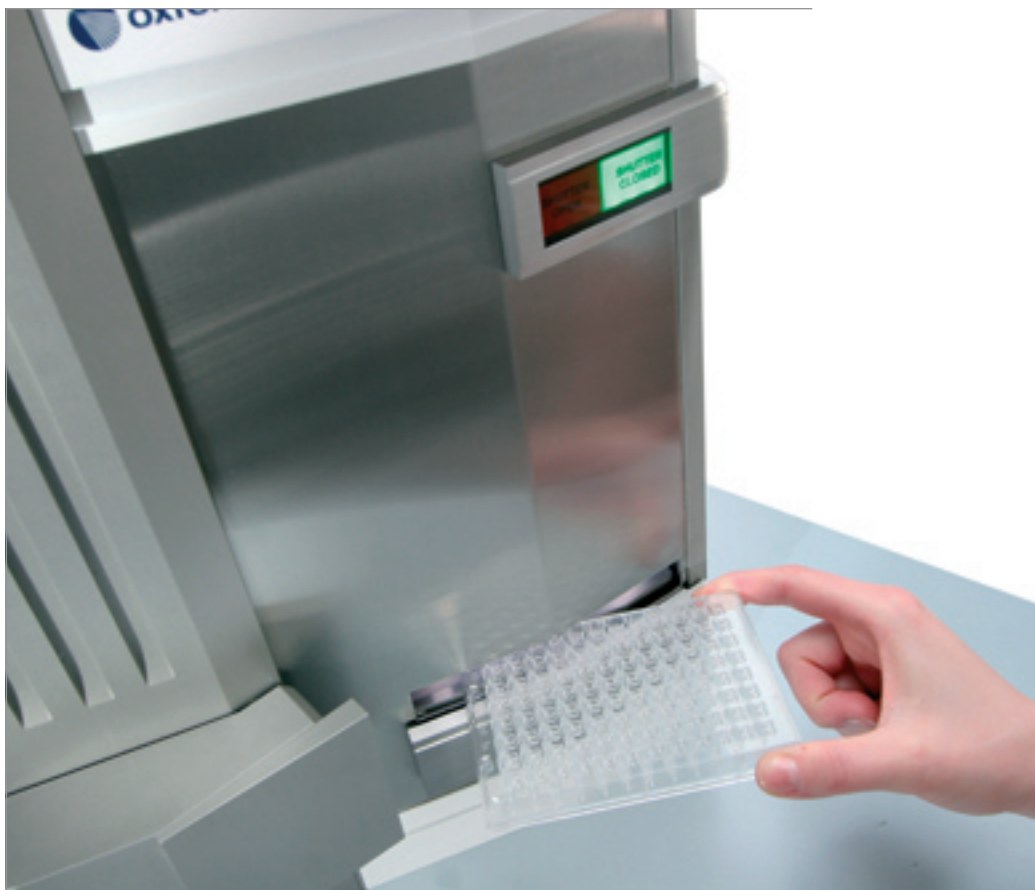
PX Scanner - Loading a crystallisation plate
