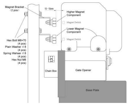
magnet should be .39 - .59 "away from the magnetic limit switch. If it is too far away, the switch will fail to work. The distance between the magnet and the opener should be 1/2" (12mm) with the opener cover on. Adjust the position of the magnet until the positions of the opening and closing meet the requirement.
