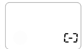
Meter Installed Backwards
