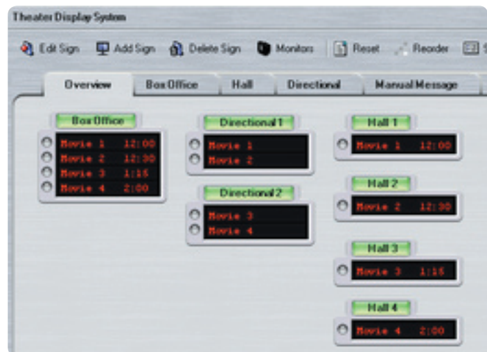
The "Overview" Tab shows all signs and their content. The signs can be arranged to simulate their arrangement throughout a theatre, or in any other convenient way.
