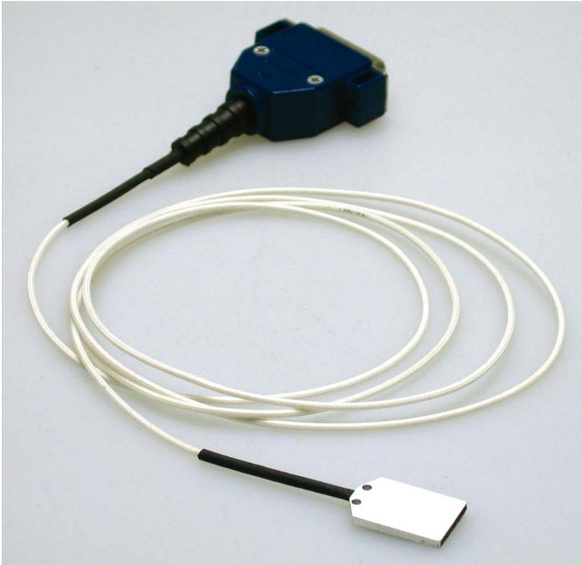
The MPA8I is a differential (type I) amplifier, that is, it includes additional **common ground** and **reference electrode inputs**. The reference electrode is ideally identical to the recording electrodes and placed into a comparable but inactive area or tissue. Background or noise signals that are picked up by both the reference electrode and the recording electrodes are removed.
