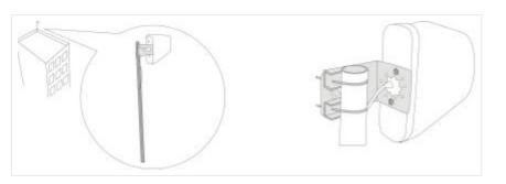
Installation of a Yaggi antenna as an outdoor antenna
