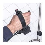
Take the flash starter handle between the thumb and the forefinger of your right hand. You can use your ringfinger or little finger to accelerate slightly during starting. With your left hand, grasp the spring on the flash starter cord
