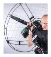
Pull the starter cord slowly until you feel resistance, until you find compression stroke, then pull quickly straight ahead. Your two arms must be stretched. After the compression stroke, your engine should start. After starting the engine, don't let the flash starter cord shoot back abruptly but let if rewind slowly. If you let go the flash starter handle abruptly, it might damage the flash starter mechanism.
