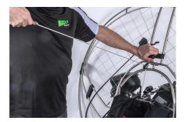
After starting the engine, you can move the choke lever to the "OFF" position after a few seconds. **Don't take off with the choke in the "ON" position !**
