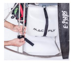
Set up the supporting arch of the upper frame, then the 2 quarters of the upper cage, without forgetting the hand starter shackle on the upper part, between the 2 cages. You can also fix this shackle to the titanium buckles welded on the upper part of the frame.
