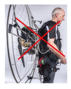
Fasten your leg straps and check that the seat board extension isn't turned under the harness, then fasten your chest strap.
