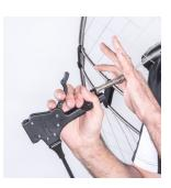
Incline the engine slightly on the right, to take easily the flash starter handle.
