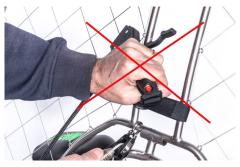
Then pull quickly and the engine should start. Reiterate the operation until the engine runs.
