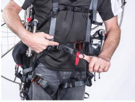
There is a small strap above the chest strap that must be closed, it only aims at preventing shoulder straps slipping during take-off and landing phases.
