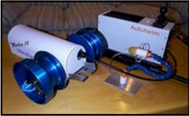
Photo 2 —A joystick or a sip-and-puff controller allows a disabled person to manage the Martin 16 Autohelm/Windlass System.
