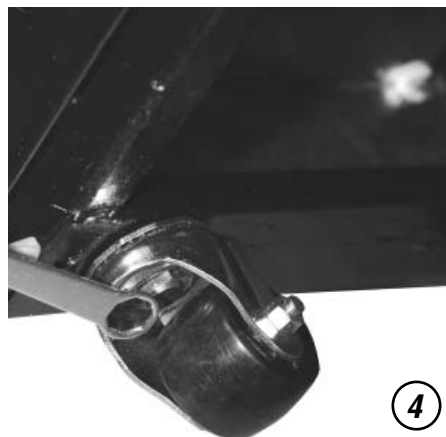
Tighten castor in position with castor wrench.
