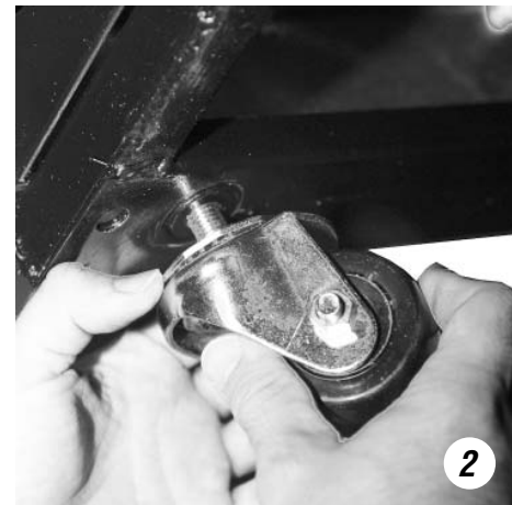
Thread castors into existing leg leveler holes.
