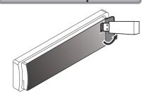
Flip open the USB plastic cover, insert the USB device into the USB socket. The unit starts playing from the USB device automatically.
