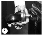
Thread castor into the underside of cabinet frame rail.
