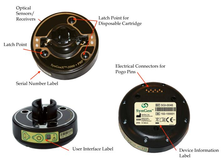
14-02-015 Revision D Effective 06/18/2015 The components of the Control Module are described below:
