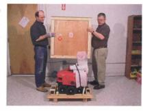
holding down the robot, and then lift the robot off the platform and place it on the floor. It takes two people to lift a CoWorker robot, with one person grasping the handles on either end.
