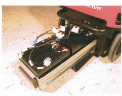
Push the battery tray back into the robot, being careful to not snag the battery cables or fuses on the inside of the robot. Next, plug in the two battery connectors to the receptacles just inside the battery access door. It does not matter which plug goes into which receptacle, and the plugs are keyed so you can only plug them in the right way.
