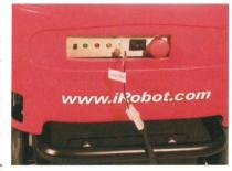
the charger. This is the so-called "remote drive-off charger cable", and it should be used between the charger and the robot to prevent the charger from being dragged behind the robot if someone neglects to unplug the robot before driving it.
