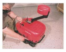
The back shell can be removed by loosening the four retaining screws and then pulling the shell straight back. Occasionally it takes a little wiggle of the shell to free it. When replacing the shell, be sure to slide the shell straight forwards, taking care to engage the shell appropriately through the volume knobs and buttons on the left-hand side speaker.
