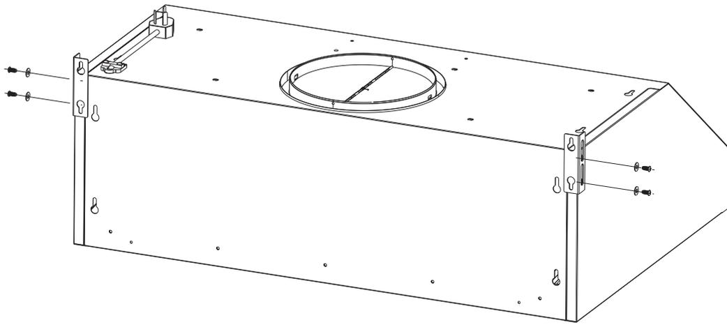
Connect the hooks, gaskets and screws to the unit by screwdriver.
