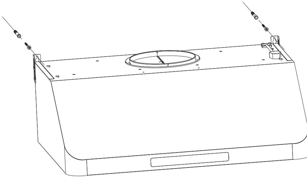
Screw the anchor screws to suitable location, then hook on, lock screws.
