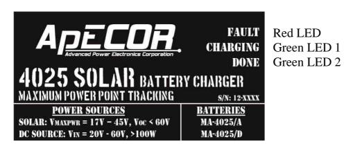
Figure 5: Label on top of charger and LED location
