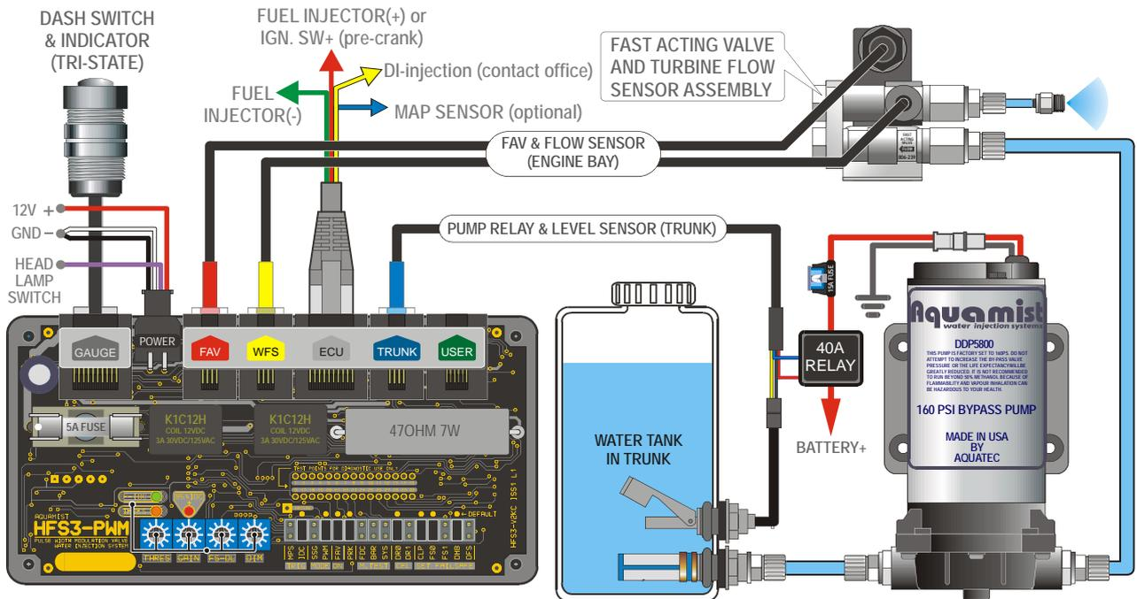
Note: Please ensure the correct harness is plugged into the appropriate socket to avoid causing permanent damage to the Electronic controller. The potentiometers on the controller are preset to mid-position from factory. System triggers at 40% of IDC. Fuel-IDC to Water-IDC ratio is 1. The system will operate correctly without any adjustments.
