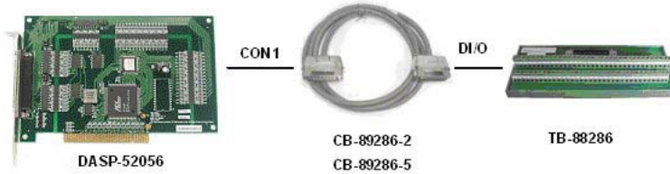
Signal Connections for DASP-52056/DASP-52056L
