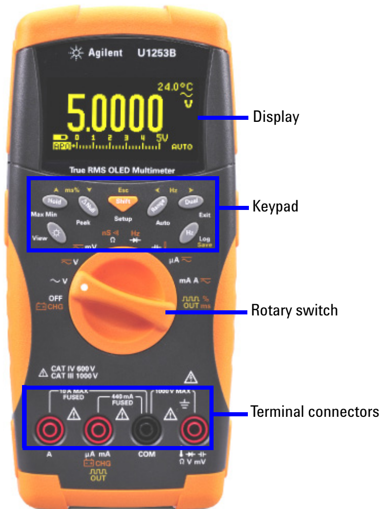
Figure 1-4 U1253B front panel
