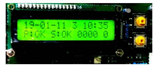
When machine is in attract mode, waiting for a customer, the upper line shows the time and date.
