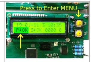
A-Insert paper in the fence and wait for the display to show P:OK, before pressing the upper button to enter the menu
