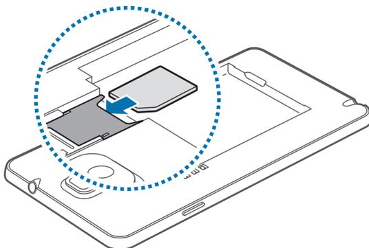
3 Push the SIM or USIM card into the slot until it locks in place.
