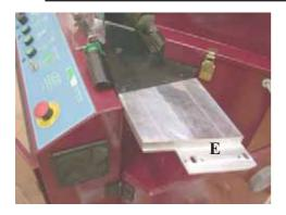
Put wedge E in place on the frame and screw it in, using the 2 frame fastening screws.
