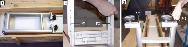
Open the crate and put the NS foot stand into an upright position. With a 4mm hex head key, unscrew the 4 screws of the 2 foot stand locking plates: P1 and P2 . Push P1 and P2 right back with a mallet, then slide them down to the bottom of each foot. Retighten the 4 screws of plates P1 and P2. With a 5mm hex head key, unscrew V1 and V2 and put the NS feet in the outside position as shown in figures 3 and 4.
