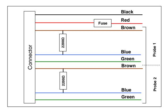
Place a 2200 Ohms resistor between the Blue and Brown wires.
