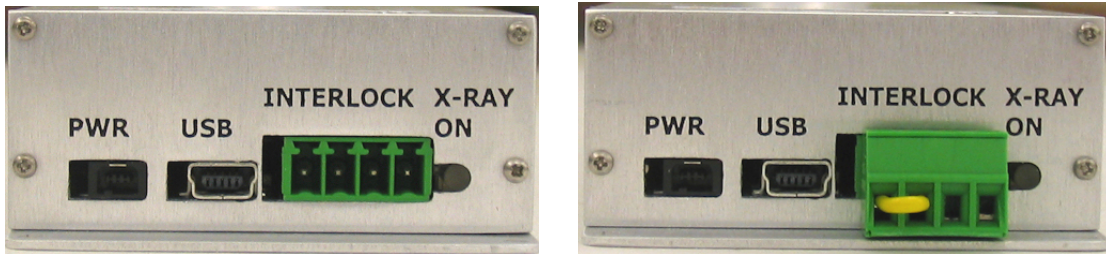
Figure 5. Showing the interlock disabled (left) and enabled (right).
