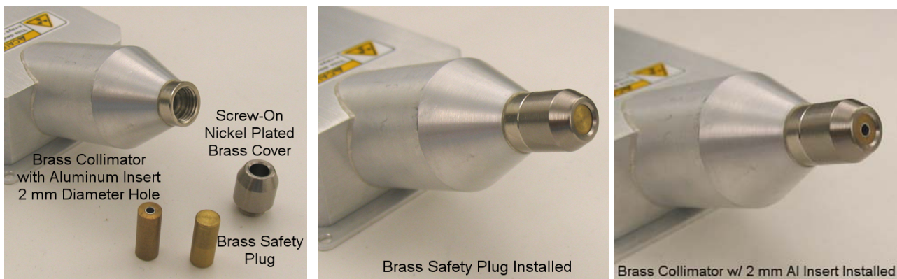
Figure 4. Left photo shows the Mini-X collimator, safety plug, and cover. The middle photo shows the safety plug installed in the cover and attached to the Mini-X. This configuration meets the radiation requirements discussed in Section 1.2. The Mini-X ships from the factory in this configuration. The right photo shows the collimator installed in the cover.
