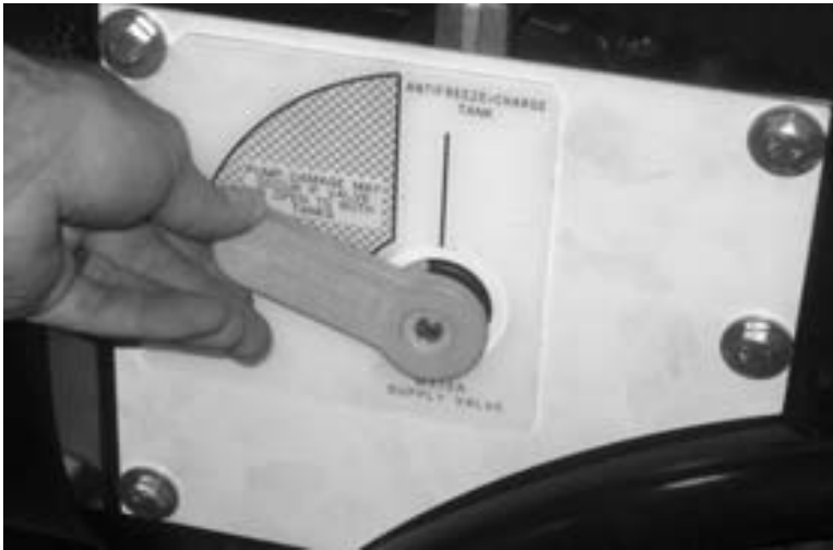
Figure 4-8. Move the Water Supply Valve to the TANKS position.
