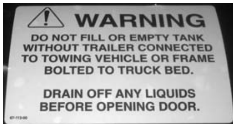
Figure 2-2. This warning label is on the vacuum filter housing. Keep the trailer connected to the vehicle when operating the vacuum system. Drain liquids through the drain valve before opening the door to dump the tank. (Part no. 67-113-00.)
