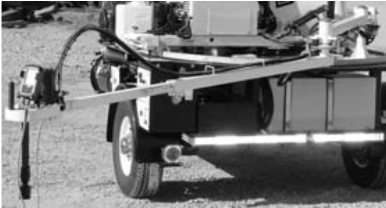
Figure 3-21. The ERV-750 valve exerciser extends on a pivoting, telescoping arm.
