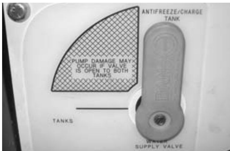
Figure 5-42. Move the Water Supply Valve to the ANTIFREEZE/CHARGE TANK position.
