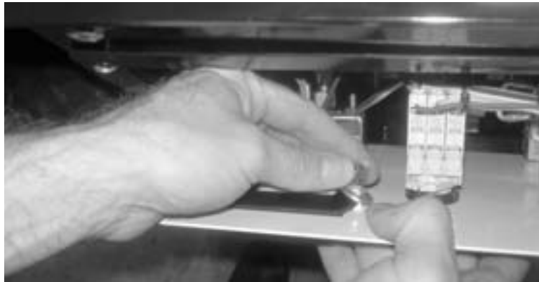
Figure 7-10. Remove the nuts and screws to take off the tach/hour meter.
