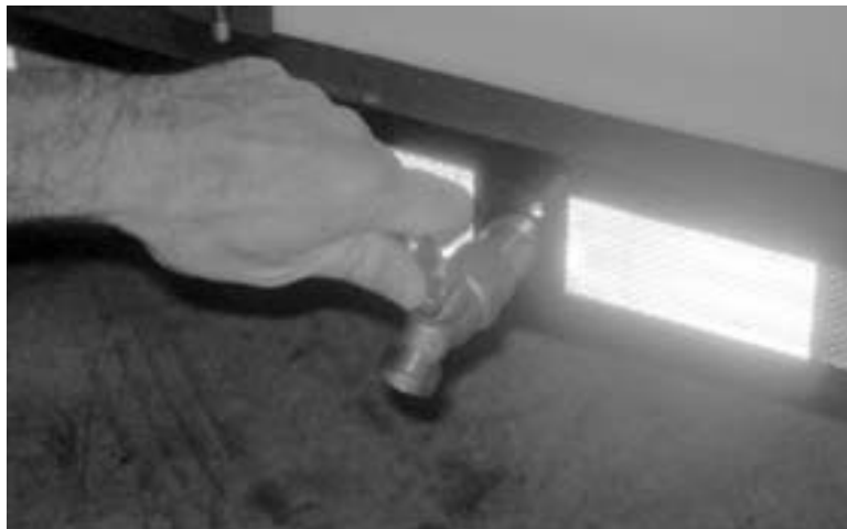
Figure 5-48. Connect a garden hose to the drain valve on the back of the trailer.
