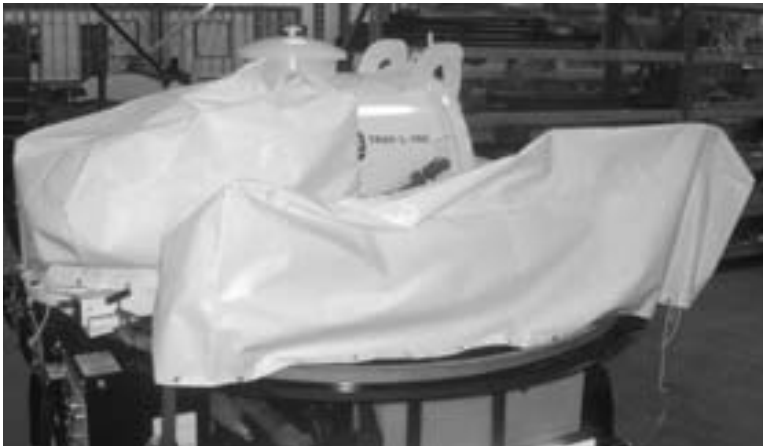
Figure 4-2. The covers supplied with the TM-7 and ERV-750 valve exercisers.
