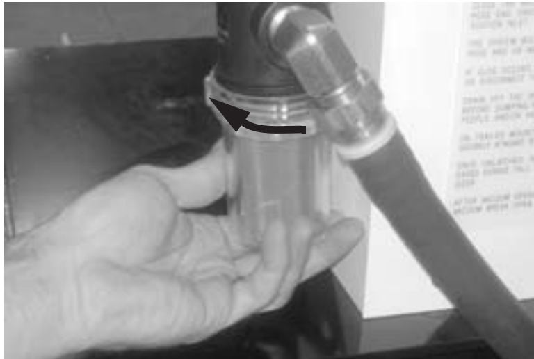
Figure 6-23. Unscrew the strainer bowl.
