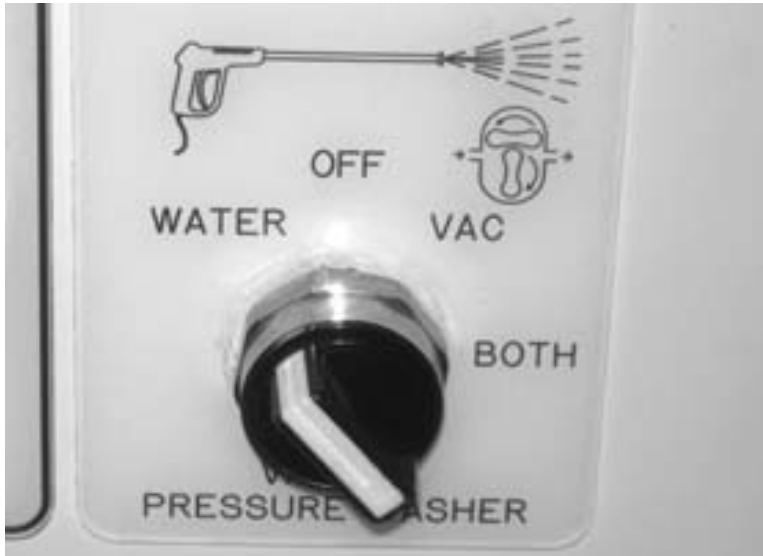
Figure 5-45. Turn the pressure washer switch to the WATER position.
