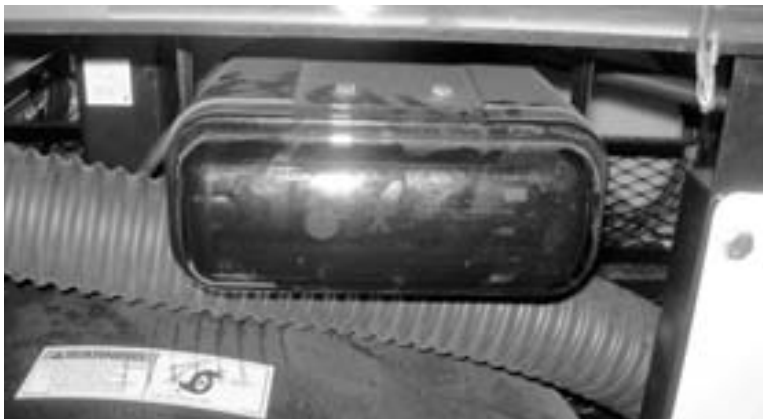
Figure 5-55. The controller for the light bar is inside a water-tight enclosure on the side of the trailer.
