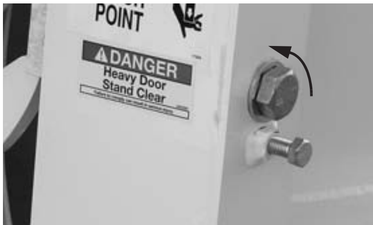
Figure 7-31. Turn the adjustment screw counter-clockwise to loosen the latch.
