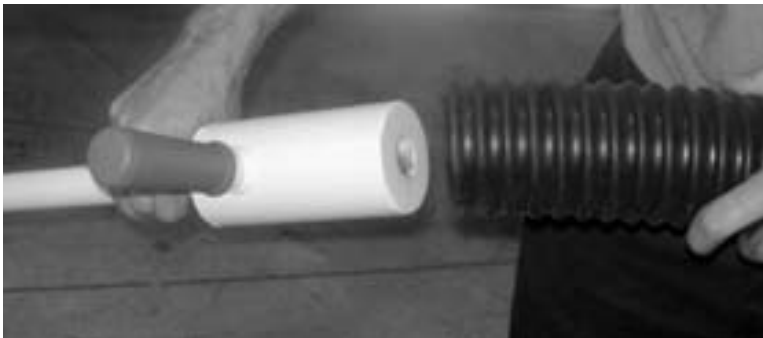
Figure 5-12. Insert the wand fitting into the end of the vacuum hose.
