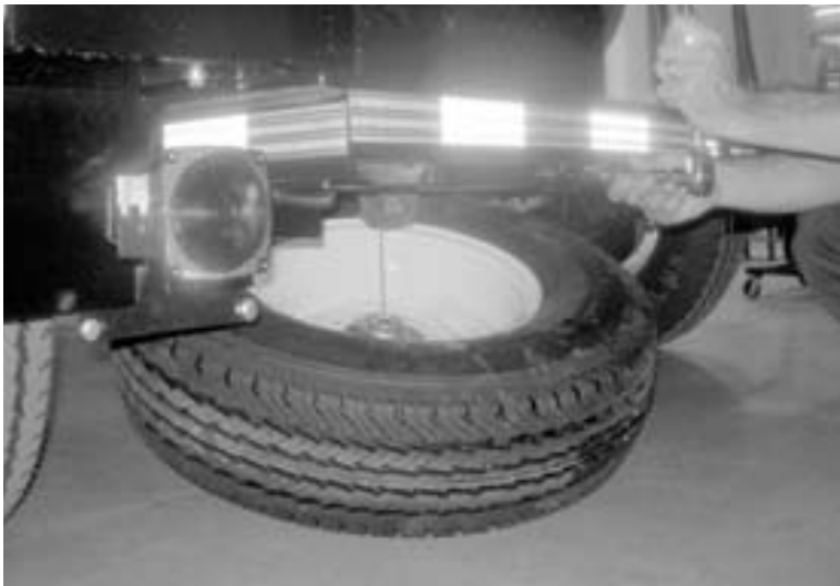
Figure 7-1. Turn the nut on the cable mount to lower the spare tire.
