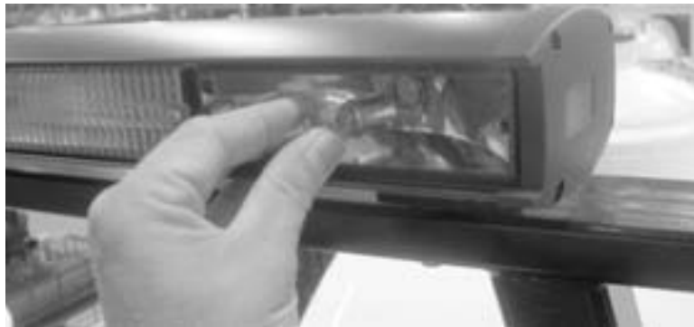
Figure 7-37. Remove the light bulb from the socket.
