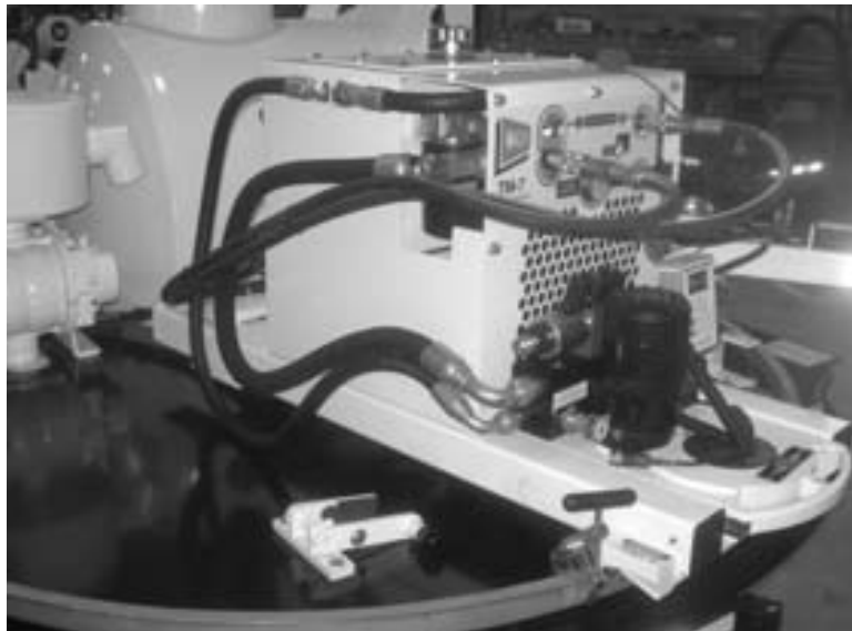
Figure 5-75. Swivel the TM-7 along the rail to the desired position, then tighten the swivel clamps.
