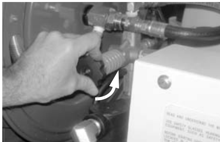
Figure 5-44. Turn the unloader knob counter-clockwise until the spring tension is released.
