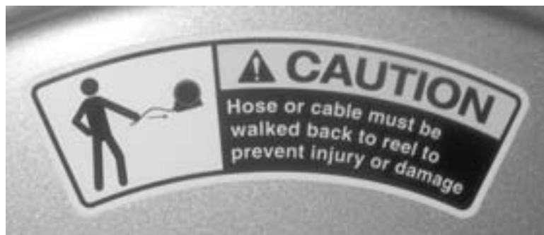
Figure 2-7. This label is on the hydraulic hose reel. When retracting the hose, walk it back to the reel. Do not let the hose snap back into the reel. (Contact the manufacturer, Cox Reels, for replacement labels.)
