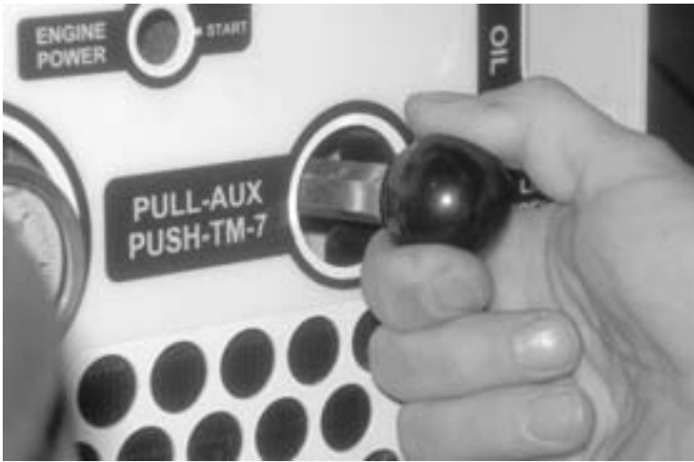
Figure 5-60. Pull the auxiliary knob on the front of the hydraulic tank.
