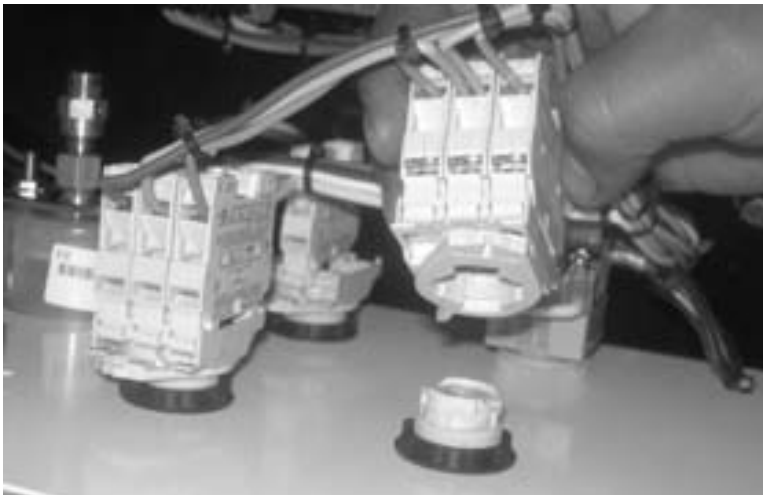
Figure 7-13. Turn the locking ring to disassemble the switch for removal.
