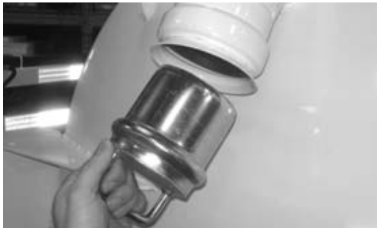
Figure 5-10. Remove the plug from the inlet port.
