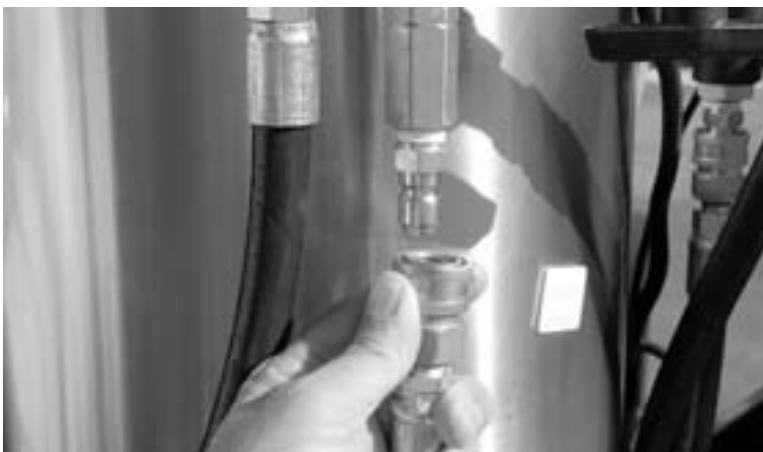
Figure 5-70. Connect the hose from the reel to the inlet on front of the water heater.
