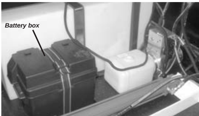
Figure 7-33. Remove the strap and take the cover off the battery box.
