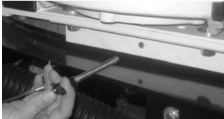
Figure 5-74. Pull out the locking pin holding the TM-7 to the frame. Replace the pin in the frame after moving the TM-7.
