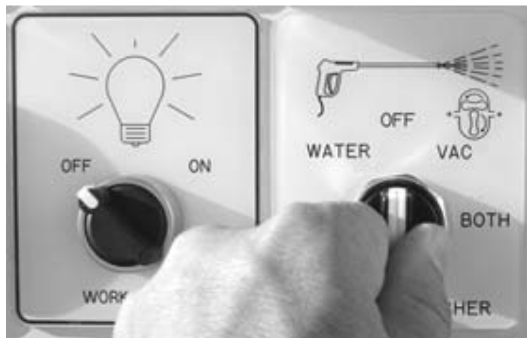
Figure 6-1. Turn the Vacuum/Pressure Washer switch to the OFF position.
