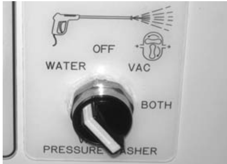
Figure 4-4. Turn the pressure washer switch to the WATER position.
