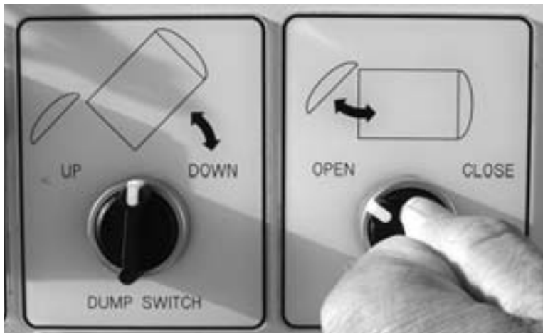
Figure 5-24. Turn the Latch Switch to the OPEN position and hold it until the door swings open.
