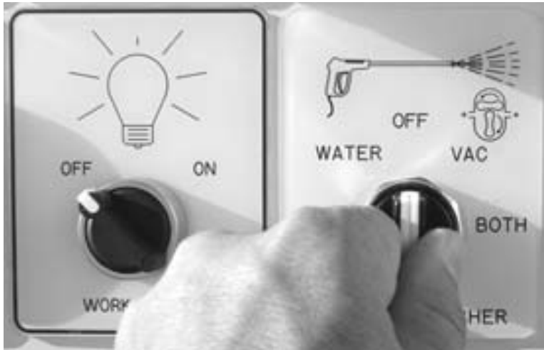
Figure 6-10. Turn the Vacuum/Pressure Washer switch OFF to turn off the vacuum.
