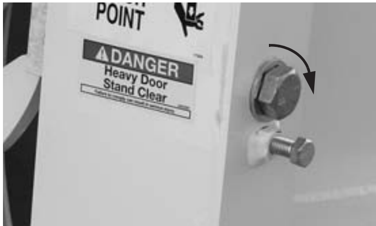
Figure 7-30. Turn the adjustment screw clockwise to tighten the latch.
