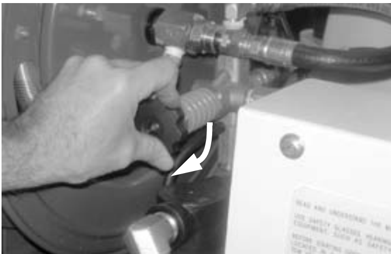
Figure 5-46. Turn the unloader knob clockwise to increase the water flow.
