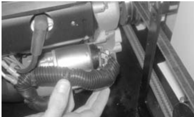
Figure 7-34. Pull back the boot on the starter motor power connector.
