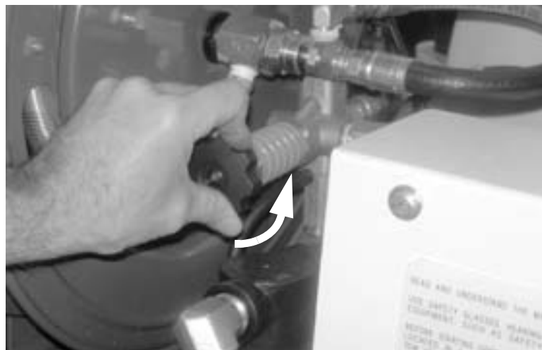
Figure 5-52. Turn the unloader knob counter-clockwise until the spring tension is released.
