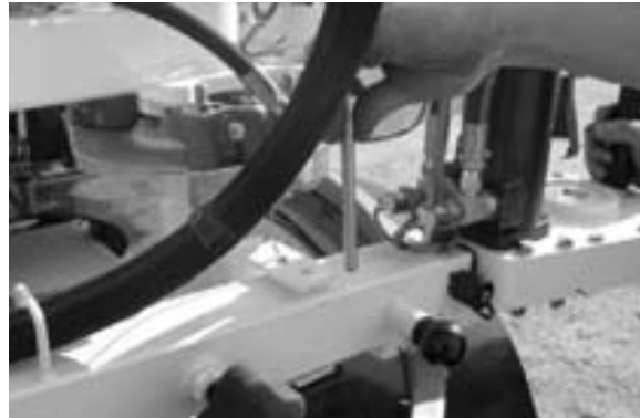
Figure 5-80. Release the two latches that secure the ERV-750 arm to the trailer.
