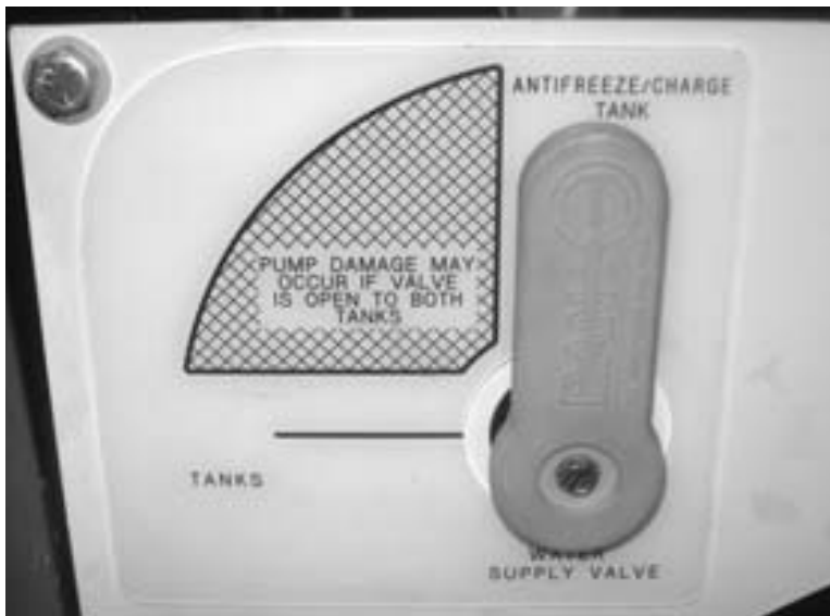
Figure 4-12. Move the Water Supply Valve to the ANTIFREEZE/CHARGE TANK position.
