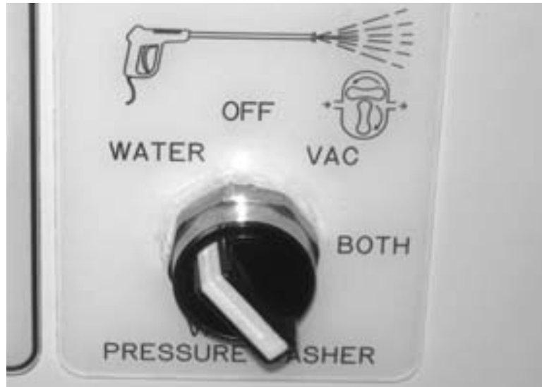
Figure 4-6. Turn the pressure washer switch to the WATER position.
