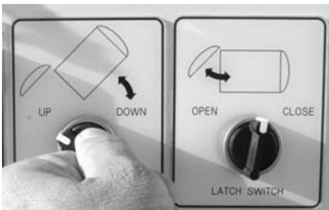
Figure 5-18. Turn the Dump Switch to the UP position and hold it just until the tank has cleared the deck and begins to tip . Tip the tank approximately 10^{\circ} - 20^{\circ} .
