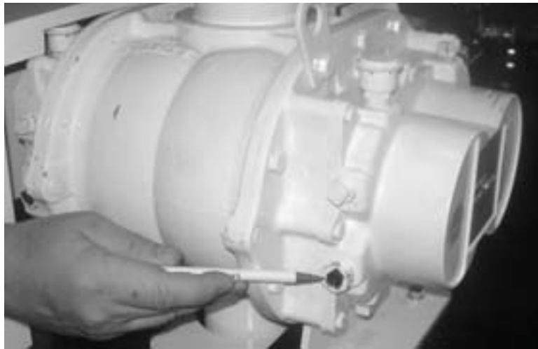
Figure 6-12. Check the blower oil level using the sight glass on the side of the blower. Oil should be visible in the glass.
