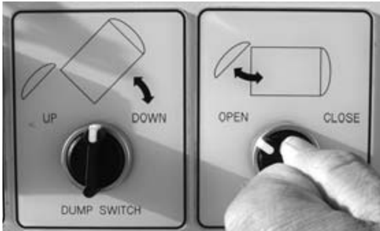
Figure 7-28. Turn the Latch Switch to the OPEN position and hold it until the latch is fully opens.
