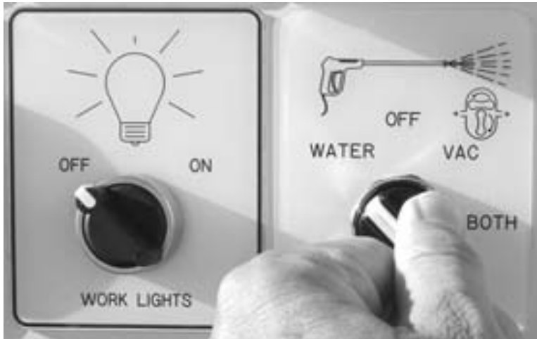
Figure 5-37. Turn the pressure washer switch to the WATER position.
