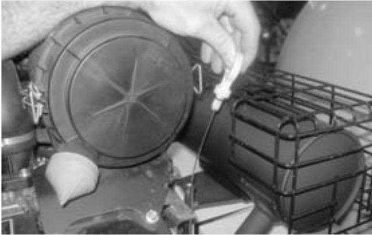
Figure 6-14. Check the engine oil level using the dipstick (gas engine shown).
