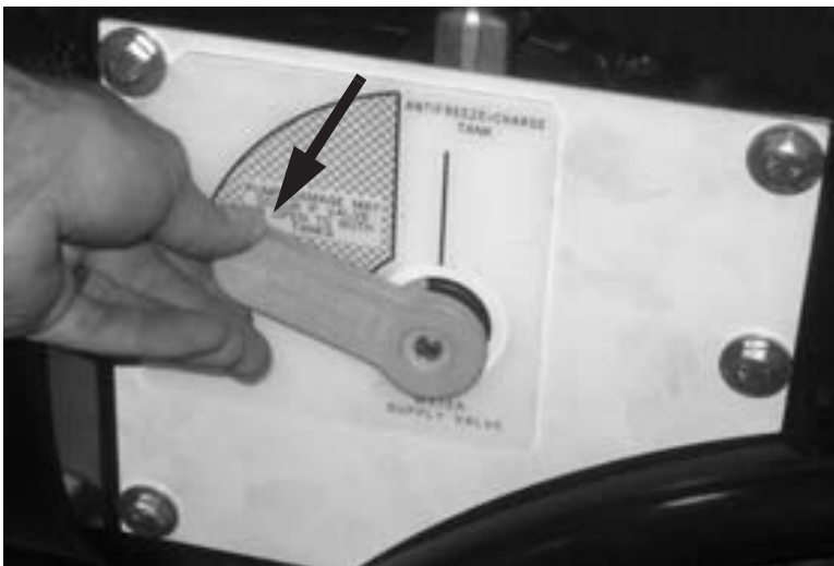
Figure 5-50. Move the Water Supply Valve lever to the TANKS position.
