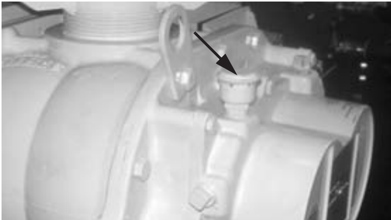
Figure 6-22. Remove the oil fill cap on the top of the blower housing.
