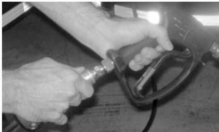
Figure 5-36. Attach the spray wand to the sprayer hose.
