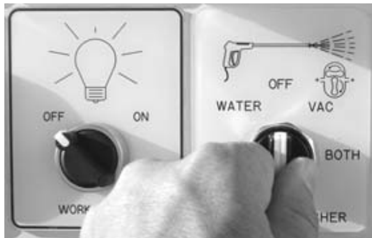
Figure 5-40. Turn the Vacuum/Pressure Washer switch OFF when finished spraying.
