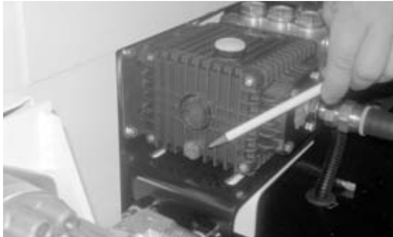
Figure 6-19. Remove the oil plug to drain the sprayer pump oil. Use a grease rag or shallow tray to catch the oil.
