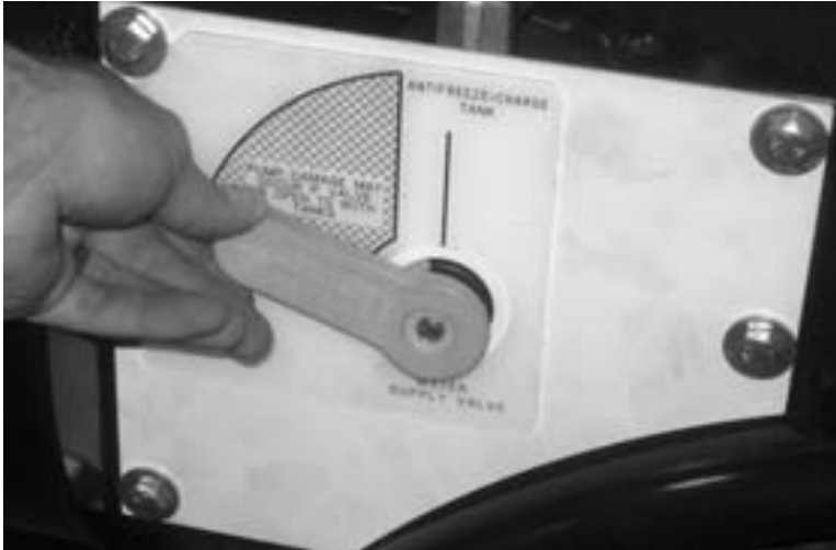
Figure 4-15. Move the Water Supply Valve to the TANKS position.
