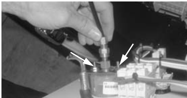
Figure 7-11. Remove the hose from the vacuum gauge, then take out the screws holding it to the bracket.
