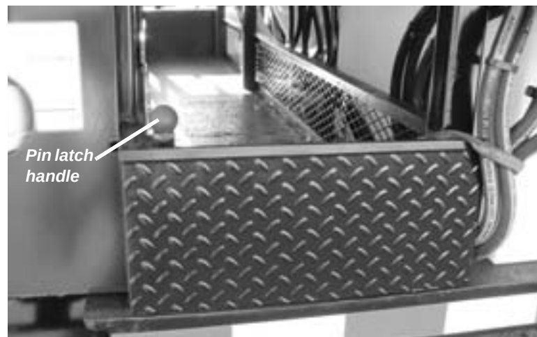
Figure 5-1. Access the storage box at the back of the trailer. Pull up the pin latch to open the door.
