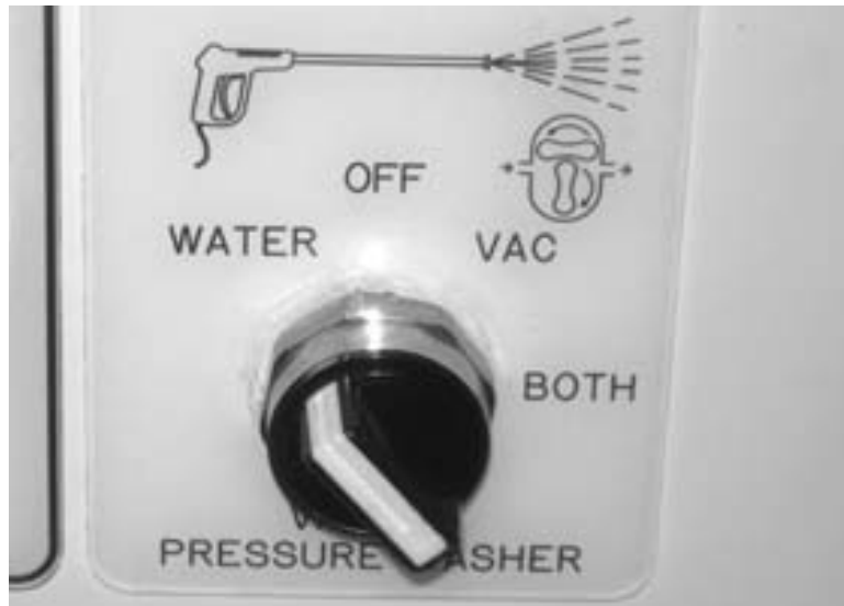
Figure 4-13. Turn the pressure washer switch to the WATER position.
