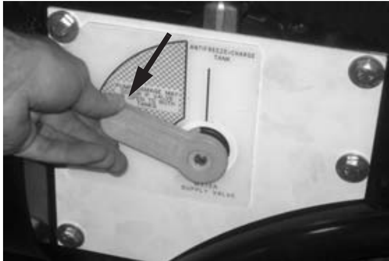
Figure 5-47. Move the Water Supply Valve lever to the TANKS position to prime the main tank.
