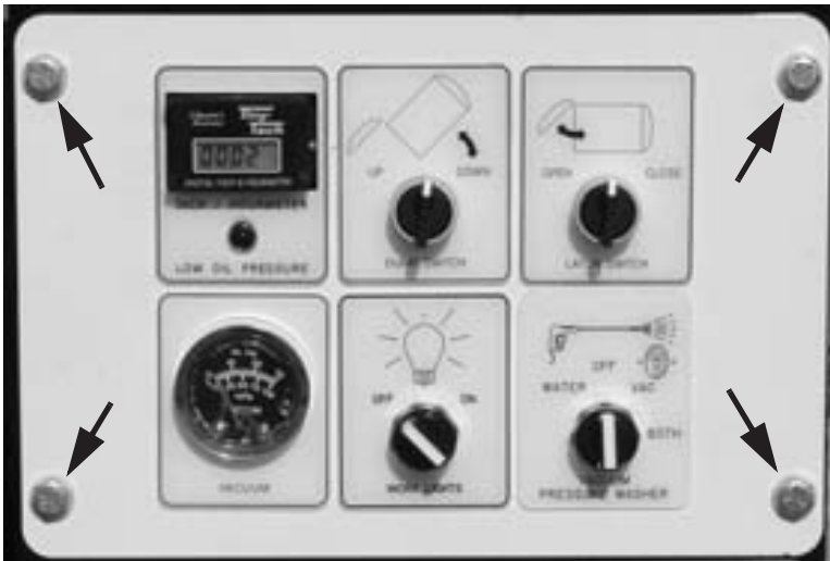
Figure 7-8. Remove the four screws at the corners to take off the control panel.
