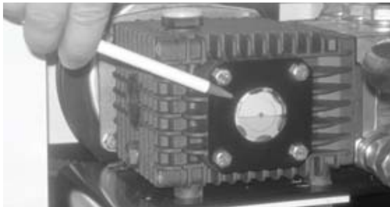
Figure 6-13. Check the sprayer pump oil level using the sight glass on the side of the pump. The oil level should be at about the middle of the sight glass.
