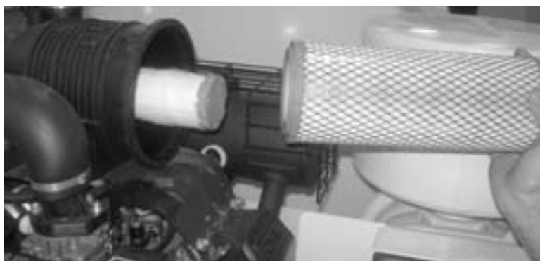
Figure 6-17. The filter has two elements. Check both and replace if dirty or clogged.
