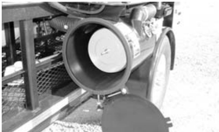
Figure 3-9. The vacuum system filter canister shown with the clean-out door open.
