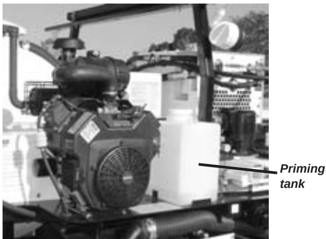
Figure 5-34. Fill the priming tank with either anti-freeze (when using the system in freezing weather) or water treated with a purifying agent (when using the system in non-freezing weather.)
