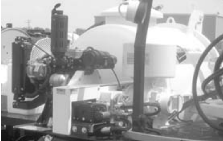
Figure 3-5. An alternate configuration is available with a diesel engine and traverse-mounted drive enclosure for the pumps.
