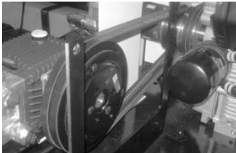
Figure 7-24. Inspect the sprayer pump belts for damage and correct tension.
