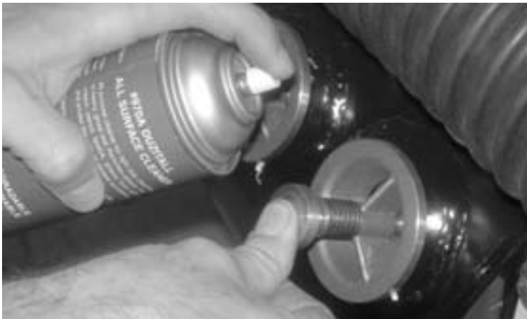
Figure 6-15. Spray lubricant on the pressure relief valves.
