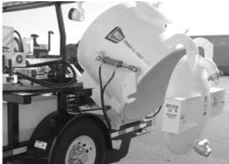
Figure 5-27. Tank in the fully tipped position.
