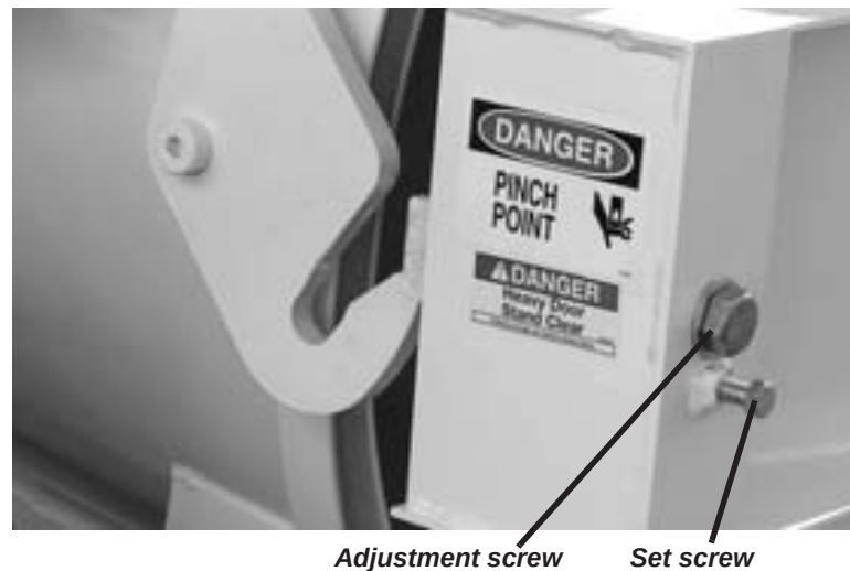
Figure 7-27. The front of the latch cover has screws for adjusting the latch.
