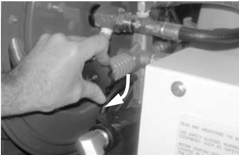
Figure 5-54. Turn the unloader knob clockwise to increase the water pressure.
