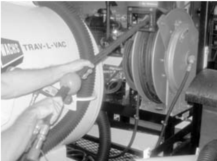
Figure 5-61. Pull the hydraulic hose pair off the hose reel to the work location.
