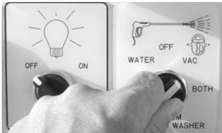
Figure 6-9. Turn the Vacuum/Pressure Washer switch to the VAC position.
