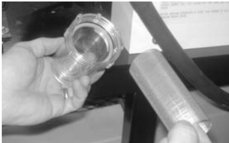
Figure 6-24. Remove the screen and clean it.
