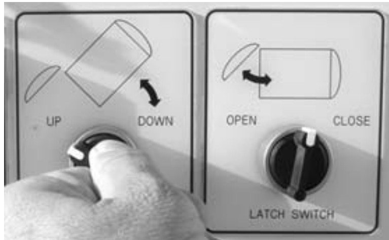
Figure 5-26. After opening the tank door, turn the Dump Switch to the UP position to completely tip the tank.
