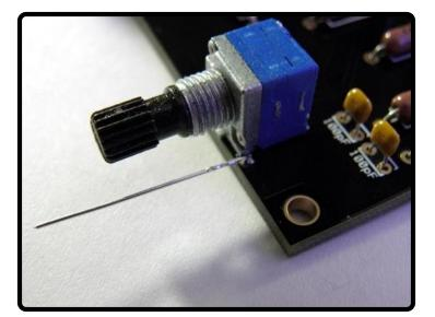
GROUNDING THE VOLUME POTENTIOMETER IS REQUIRED AS WITHOUT IT, THE AMPLIFIER MAY BE SUBJECTED TO NOISE / INTERFERENCE.
