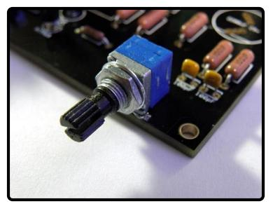
PUT ON WASHER AND NUT INCLUDED IN THE KIT. ONCE TIGHT, THE VOLUME KNOB MAY BE INSTALLED.
