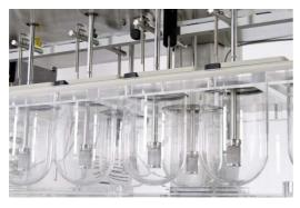
Motorized Sampling System EPE-1210 which lowers and rises the sampling ferrules into the media and after sampling back out again. 10 different sampling positions can be programmed. ITM-1210 Media Temperature Monitoring system which is attached to the EPE-1210 will read and report the media temperature while sampling. And a manual or motorized Tablet Dropping Magazine TM/TMA-1210 with its attached low evaporation vessel sealing covers complete the set of useful accessories for automation.
