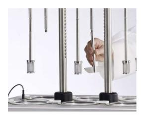
The PTWS D610 uses the Pharma Test MonoShaft™ design. Tools consist of the main shaft plus interchangeable tool heads (adapters). The main shaft remains in place in the instrument regardless of the tool head being used. The clearance of each tool from the vessel base will always be correct once the main tool shaft has been installed and fixed in its position.
