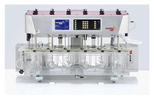
The PTWS D610 is Dual-Drive 6 + 6 stirred position tablet dissolution testing instrument for solid dosage forms as described in USP chapter <711/724> and EP section<2.9.3/4> as well as the DAB/BP and Japanese Pharmacopeia section <15>, having 2 extra beakers to take media refilling and reference standard media. The PTWS D610 is the ideal choice for Bio-Waiver studies and Dissolution Method Development.
