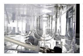
The U-shaped water bath rests on vibration absorbers to avoid any vibration transfer from either inside the instrument or even from external equipment placed on the same bench surface. The bath cover can also be easily unscrewed for cleaning. The water bath contains a water diffuser for faster heating and to ensure that heated water is evenly distributed throughout the whole bath.
