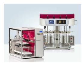
It is also possible to use the DSR-M dissolution sampling robot which features the capability of sample dilution and media refilling. The DSR-M offers excellent sampling and refilling accuracy via the fully integrated valve-less piston pump module. Sampling time and interval control is programed the PTWS D610 while volume, dilution ratio and refilling option are set at the DSR-M instrument.
