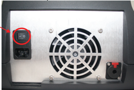
Figure 8: Main Power Switch Location
