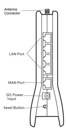
LAN Port: Four local Ethernet ports for connecting the local computers
