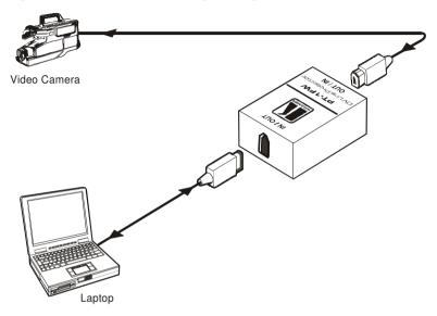
Figure 2: Connecting the PT-1FW DV Line Protector
