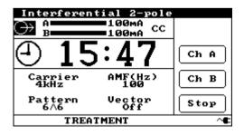
Pressing this causes both outputs to smoothly reduce to zero over a period of 5 seconds.
