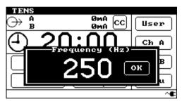
The pulse frequency may be set from 1 to 250 Hz in 1 Hz increments by pressing the numerical digits and then pressing OK.
