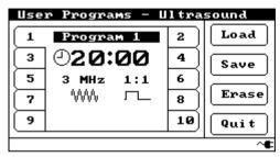
The LCD shows the 10 user programs as file cards with numbered tabs. To select a program card just touch its tab.
