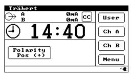
The available options are treatment time, polarity and CC/CV. These are set in exactly the same way as in the other operating modes.
