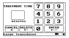
Type in the desired time and press ENTER to return to the main screen.
