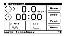
Touch the screen on the digits of the time display to increment some treatment time (maximum 30 minutes). Alternatively, touch the clock symbol to bring up the following screen:-
