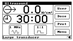
Select the desired ultrasound Frequency and Mode (pulsed or continuous) by touching the relevant field on the screen.
