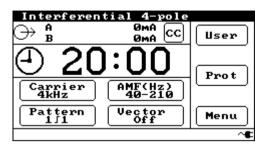
*Treatment time:* Is selected either by touching the digits of the time display or by pressing the clock symbol and entering the desired treatment time. The time can be set in 30s intervals.
