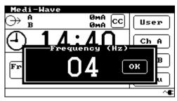
The frequency may be set from 2 to 60 Hz in 1Hz increments.
