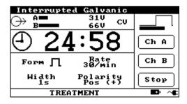
CC/CV: The output may be set to be constant current (CC) or constant voltage (CV).
