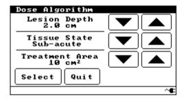
The data concerning the state of the area to be treated is chosen using the Up/Down buttons, then pressing Select will cause the algorithm to calculate the relevant treatment settings.
