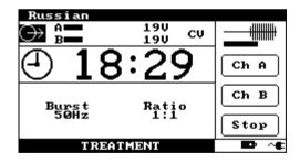
*CC/CV:* The output may be set to be constant current (CC) or constant voltage (CV) by pressing the CC/CV button. In constant current mode the electrode impedance is monitored and if the impedance for either channel is too high then the output is terminated and an alarm sounded. In constant voltage mode, if the electrode impedance rises then the output current is automatically reduced.
