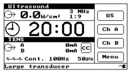
Note that two independent buttons for Ch A and Ch B now appear at the right of the screen, reflecting the fact that independent channel level control is available for all stimulation modes except 4-pole interferential.
