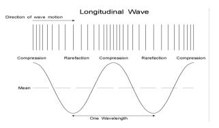
The diagram shows a sound wave travelling from left to right. The vertical bars represent thin slices of the medium which are displaced to form areas of compression and rarefaction. The sine wave represents their displacement relative to their mean position. The distance over which the vibration repeats itself is called the wavelength. The number of complete vibrations in one second is called the frequency of the sound wave.
