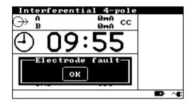
When a constant current output is chosen and the unit is operating in 4 or 2 pole interferential, russian, diadynamic, sinusoidal, galvanic or träbert modes, the electrode impedance is monitored to ensure that adequate electrode contact is maintained.
