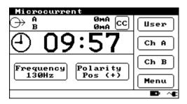
*Freq:* The frequency may be set from 1Hz to 1000Hz in ascending jumps by repeated presses of this button.
