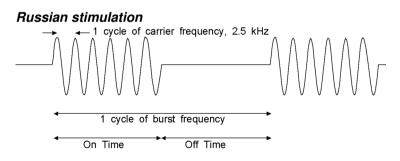
The burst frequency may be set to be from 1 Hz to 100 Hz. The on and off times are always equal and are from 0.5s (1 Hz burst) to 5 ms (100 Hz burst).
