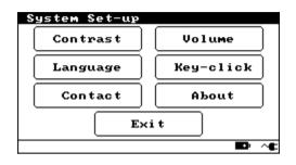
The Contrast button takes you to a screen where you can adjust the display contrast using up/down buttons.
