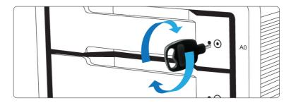
2 Insert the drive pin into the pin release until the handle of the drive module pops open.
