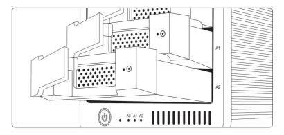
Insert the new drive in the same orientation as the drive you removed. The key holes should be on the same side as the drive labeling. Push the drive in all the way and then press in the drive module handle until it locks securely into place. Please do not use excessive force to insert the drive or you can damage it. The new drive will mount onto your OS.
