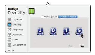
6 Check all of the drives that you would like to include in the RAID set and select "create". Drives are numbered from top to bottom (A0 top, A1 middle, A2 bottom).
