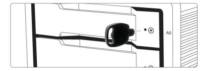
3 Pull the drive module from the T3 enclosure.
