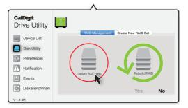
4 Go back into the "Disk Utility" tab and select "Create New RAID Set". Select the RAID mode you would like to create.
