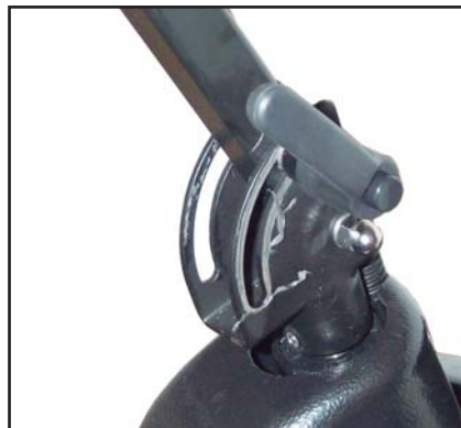
Adjusting the angle of the handlebars.
