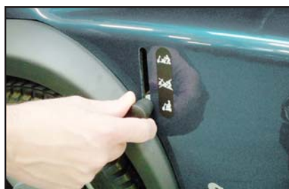
Turn the knob on the freewheel lever anti clockwise to remove it.
