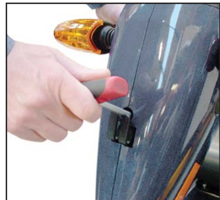
Adjusting the height of the handlebars.
