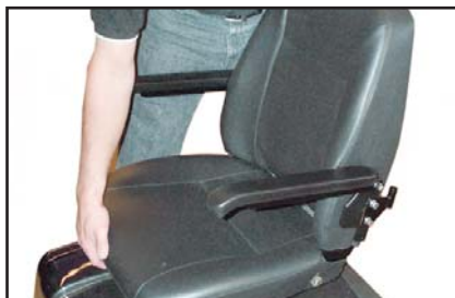
Lift the seat off the seat tube.
