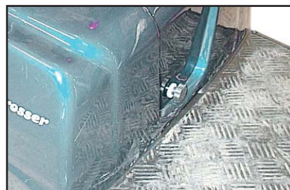
Turn the finger screw on the front of the rear shroud anti-clockwise, and remove it.
