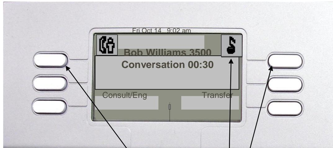
To switch between calls press the 1<sup>st</sup> white button on the left or the right. The button on the right is your 1<sup>st</sup> caller and the button on the left is the 2<sup>nd</sup> caller. Each time you press one of the buttons your current caller is automatically placed on hold. See the musical note.
