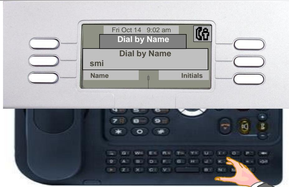
Use the Alphabetic keypad to dial by name. Enter at least 2 characters of the last name of the person you want to call, then press the button next to Name on the display. When more than one name meets the entered criteria, use the Navigator Down Arrow key to scroll thru the names. Press the button next to the person's name you wish to call.
