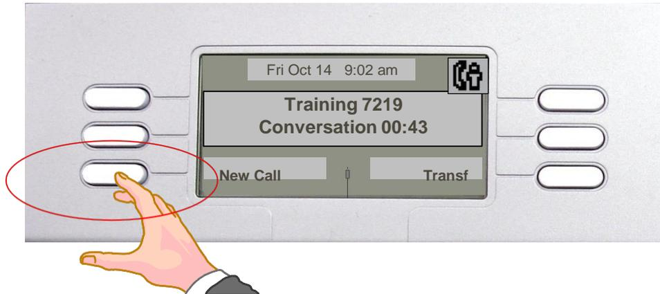
Press the **New Call** key (1st caller will automatically be placed on hold), Dial the number where the call will be transferred.
