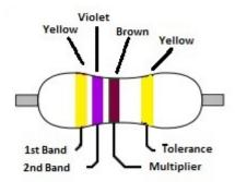
Note: Either yellow and Gold will denote 5% resistor tolerance when used as the tolerance band.
