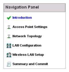
A green checkmark to the left of an item in the **Navigation Panel** defines the task as having its minimum required configuration set correctly. A red X defines a task as still requiring at least one parameter be defined correctly.
