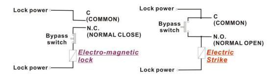
The maximum switching voltage of the relay is 120VAC or 60VDC, and the maximum switching current is 2A.It can be used to connect to the bypass switch of an electric strike for door access controlling. Overloading the maximum ratings may cause damages to the reader permanently and cannot be repaired anymore.
