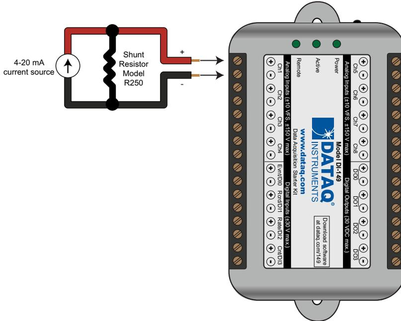
The shunt resistor should be placed on the low side of the circuit as shown below:
