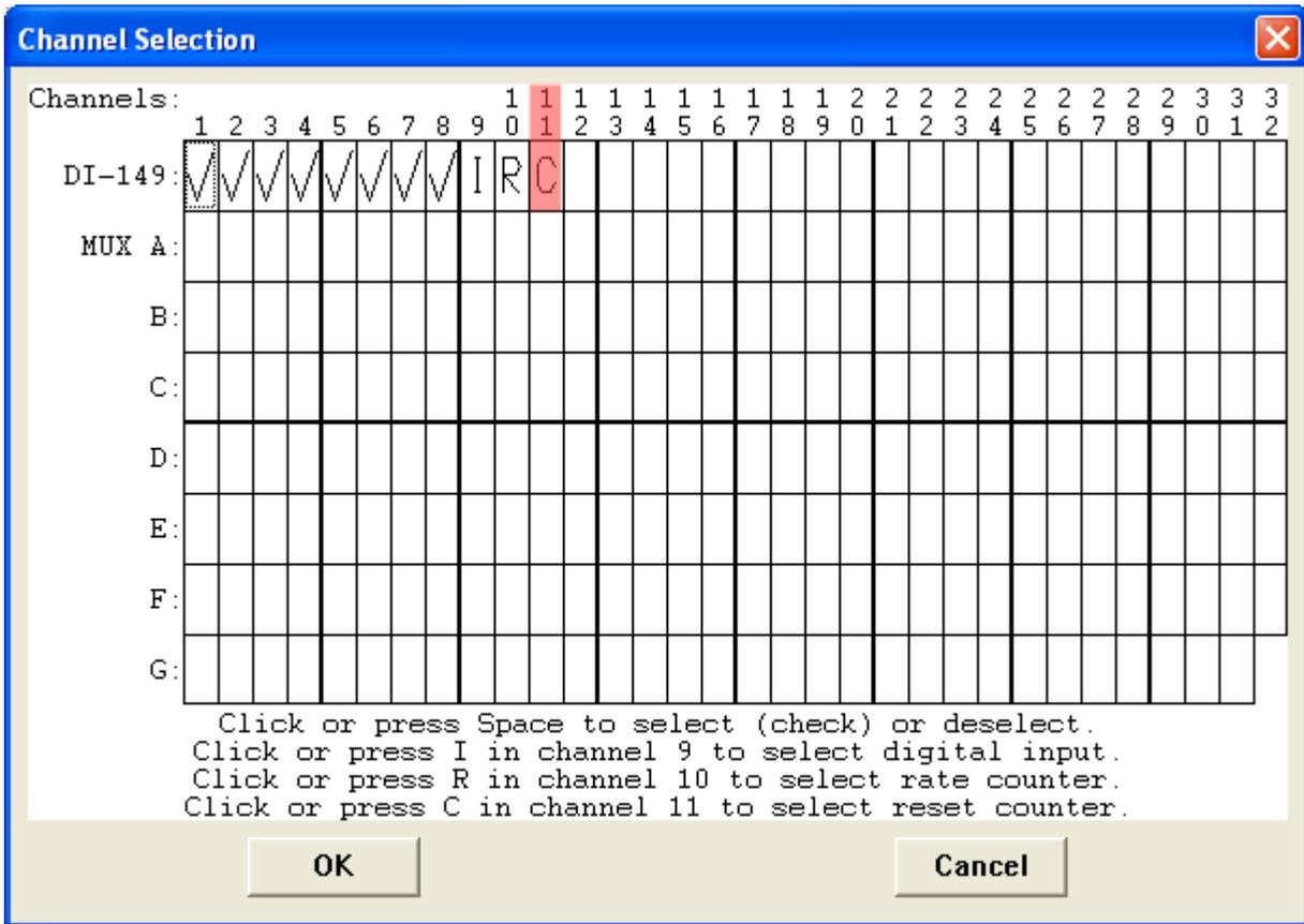
The counter channel accumulates counts over time whether recording or in standby mode as soon as the Counter channel is enabled. The *accumulated* values will be recorded to your data file unless you reset the counts to zero. The maximum count value is 16383 before the counter resets to zero automatically.
