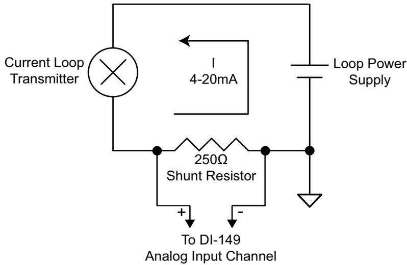
Set the engineering units as desired and define low/high calibration values in WINDAQ as 1V = 4mA for the low value and 5V = 20mA for the high value. For example, when using WINDAQ Acquisition software, in the Channel 1 Low Calibration dialog box:
