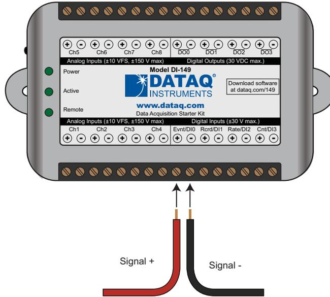
Once the switch closure or TTL signal is connected, activate Remote Events through WINDAQ Acquisition Software. Events may be automatically placed on the rising or falling edge of the trigger signal. Use the menu command **Options > Remote Events +** to set WINDAQ to place event markers on low-to-high transitions of the Event input. Use the menu command **Options > Remote Events -** to set WINDAQ to place event markers on high-to-low transitions of the Event input.
