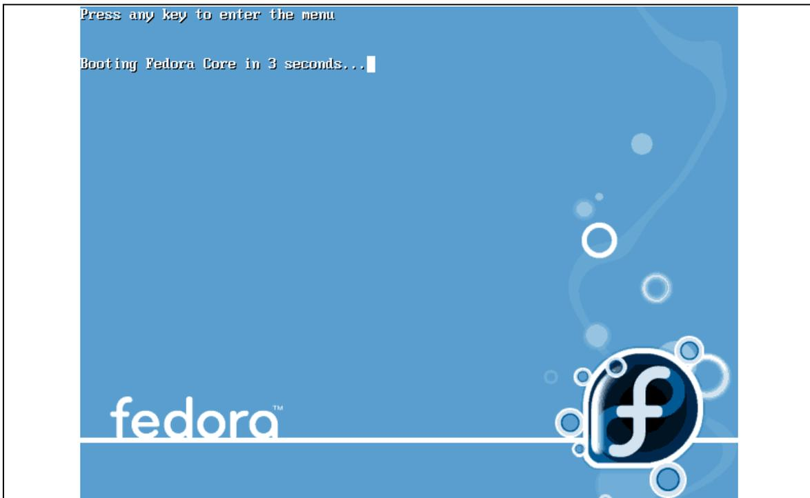
4. When a blue screen with the text “Press any key to enter the menu” appears, quickly press any key on the keyboard. If you do not press a key within time, the ALDM will boot normally. If this happens, power cycle the electronics console, or press the “CPU Reset” button on the back of the ALDM electronics to try again.
