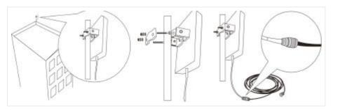
Installation of a wide directional antenna as an outdoor antenna
